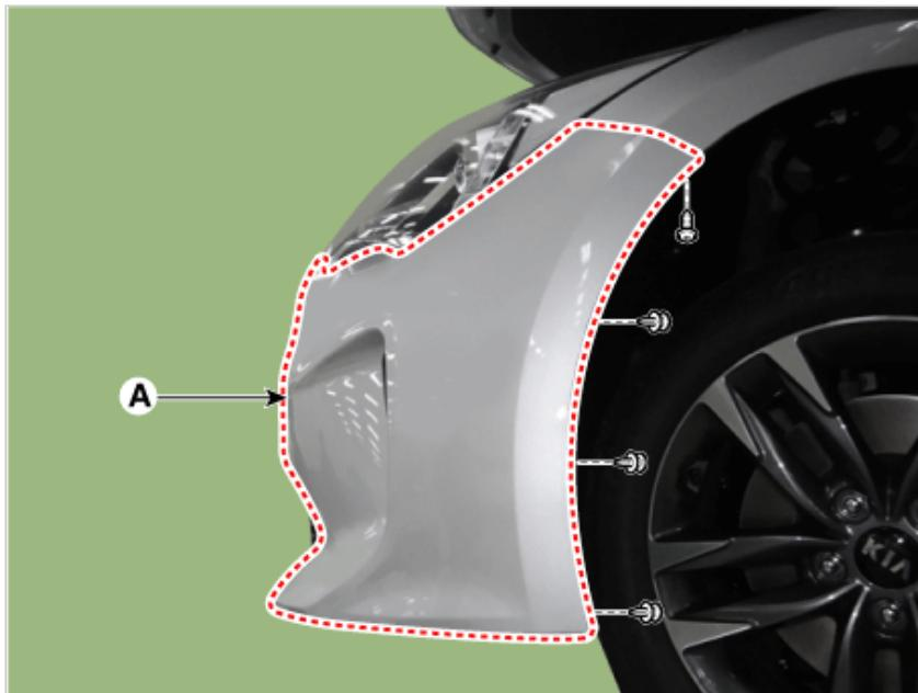
5. Disconnect the front bumper main connector (A).
