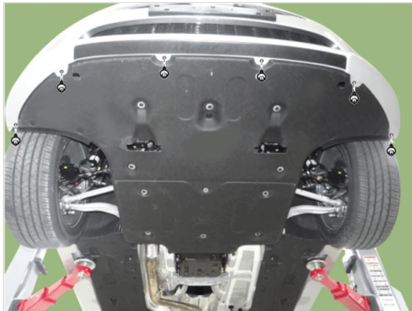
4. Separate the front bumper (A) after loosening the sides mounting clips and screws
