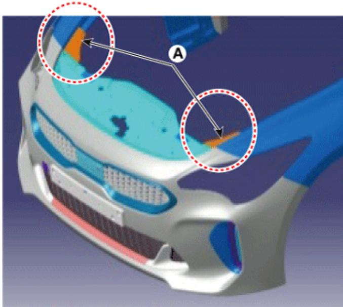
2. Loosen the radiator upper cover mounting clips and sides mounting bolts.
