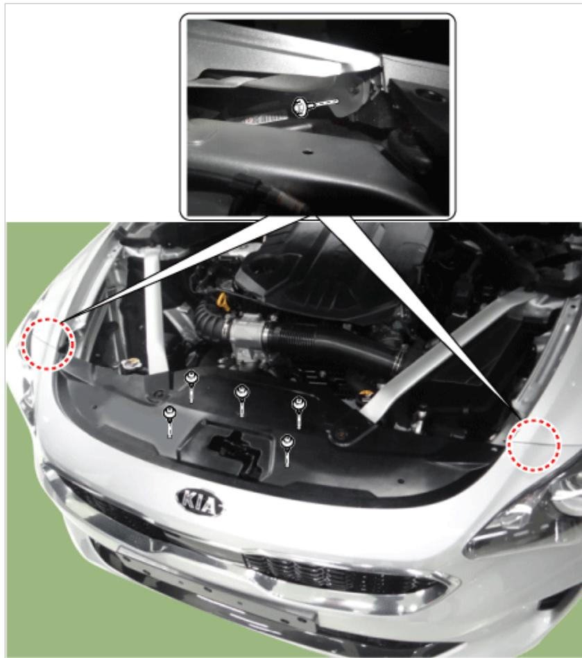
3. Loosen the engine room under cover mounting clips.
